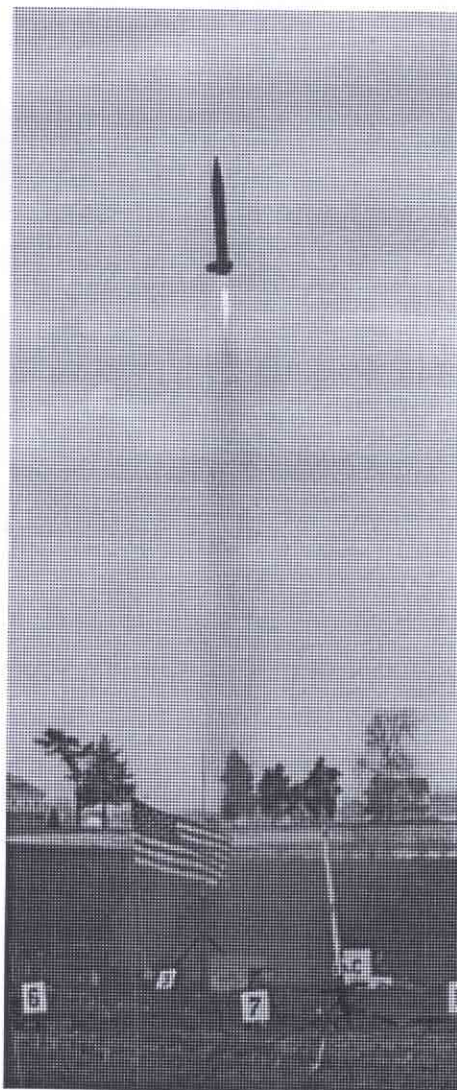
Guy DeStefano's I-ROC moves quickly off the pad on an I357T. (Brust)
